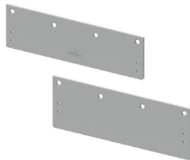
1450-18PA / 1450-18PAFC Plate Required for parallel arm mounting where top rail is less than 4 3/8" (111mm), measured from the stop Requires 1 3/4" (44 mm) minimum top rail With full cover, use plate 1450-18PAFC
