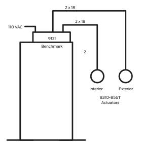
Operation: No latching at this door. For a single occupancy restroom. Either actuator will open door at any time.
